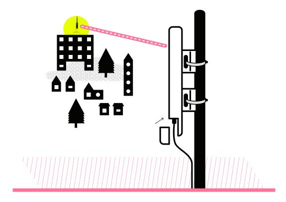
If possible, face the indicator lights on the node towards the street or ground, so they are visible without climbing onto the roof. This can help with troubleshooting in the future.
